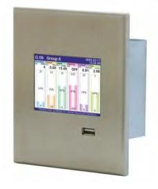
Panel or in-wall mount Multi-Channel KBL-99SL is featured by a shallow casing - only 55 mm! All connectors are introduced on side walls of the device as in a typical panel computer. As the number of measurement inputs and outputs is limited, this design in intended mainly for systems with a small number of signals or systems which include other measurement systems with Modbus RTU interface. An Ethernet interface is also available to upgrade every Multi-Channel control's application easily.
