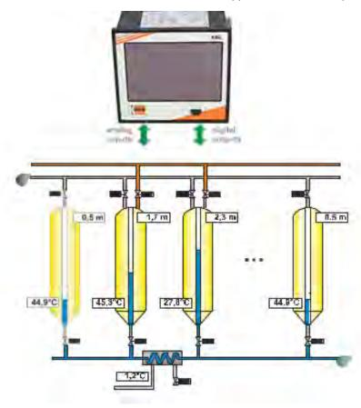
In this kind of industry application KBL-99 collects all analog measurements and sends them through Modbus RTU to main PLC. The distance between KBL-99 and a PLC installation can be up to 1000 m. All measurements are sent using one cable, this is a very cost effective method. Modbus RTU is very popular and reliable communication protocol. There is a possibility to divide Modbus network into several subnets. KBL-99 can work as a Master in one subnet and as a Slave in another.
