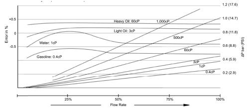
Pressure Drop Curves for Standard and Special Cut Rotors (option "S") in %age of max. Flow
